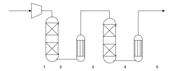
1 compressor 2 oil-removal tower 3 temperature adjustor 4 dehydrogenation tower 5 cooler
