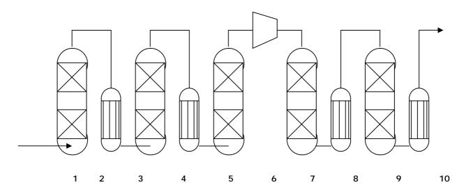
1, 2, 3, 4, 5 ATFSR unit 6 compressor 7 oil-removal tower 8 temperature adjustor 9 dehydrogenation tower 10 cooler
